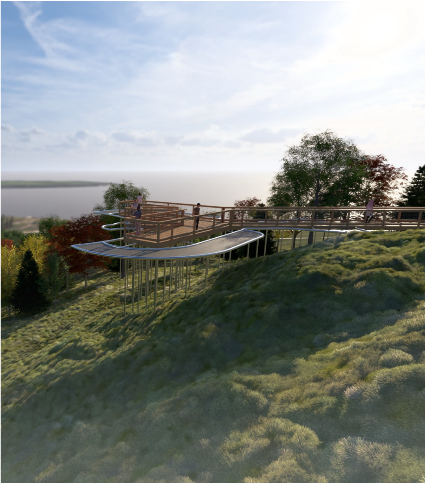
Side view of Soaring Eagle Vista showing an elevation of approximately 7 metres from the ground to the deck floor
